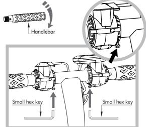
Adjust and fix the throttle and electric brake with small hex key provided.
