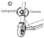
• Turn the locking knob clockwise and fasten tight the steering column.
