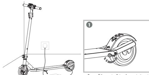
Power off the scooter. Set up the scooter in rest mode and let it rest on ground and open charging port cover.
